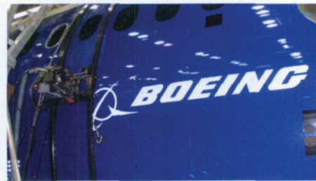
图1 应用于787机身段对接区的柔性导轨自动制孔设备 Fig.1 Flexible track automatic drilling equipment for docking area of Boeing 787 fuselage
