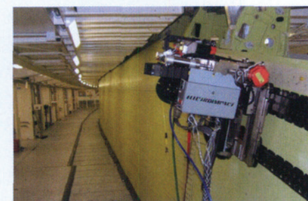
图3 应用于A380主翼盒的柔性导轨自动制孔设备 Fig.3 Flexible track automatic drilling equipment for A380 main wing box
